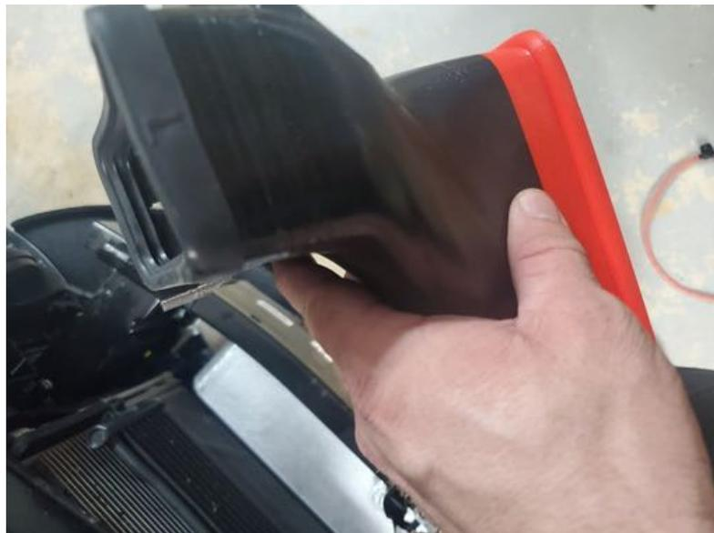
2. Push the air scoop onto the rectangular pass-through where you removed the OEM attachments. Use 2 bolts for the OEM attachments to secure the air scoops. Tighten
