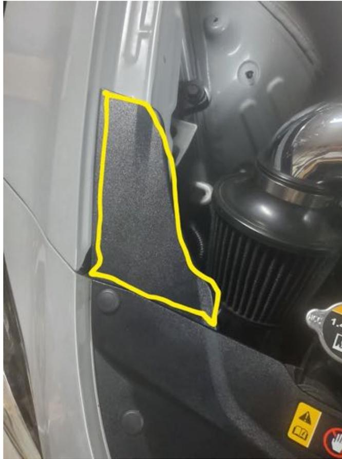
3. Using ratchet and 10 mm with short extension remove the bolts on each side
