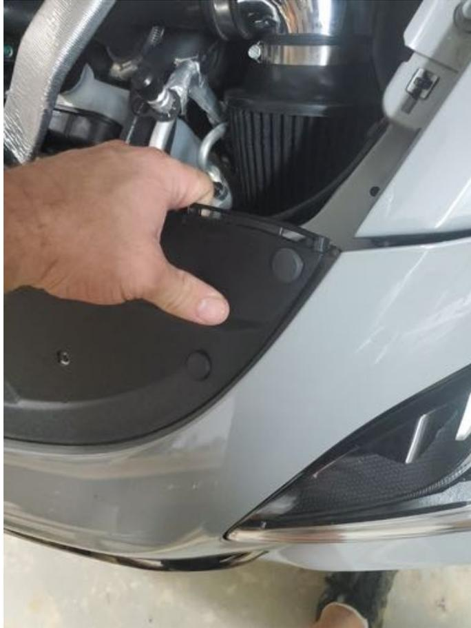
7. Disconnect wiring harness by pulling the tab on the right side
