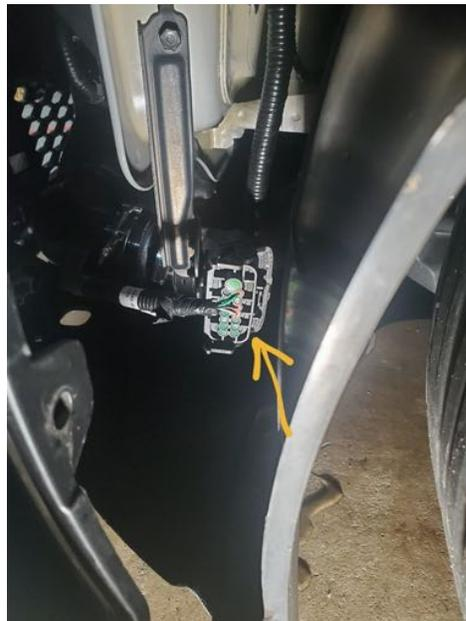
8. Pull off the front by pulling the black piece in the engine bay up and over the hood latch and then pulling the front away from the car. Set front aside in a safe location.
