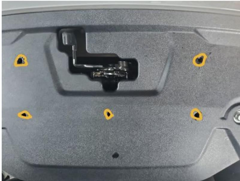
5. Remove the 6 push tabs on the underside of the bumper
